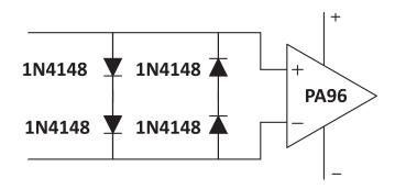
If experimentally optimizing the compensation capacitor, turn off the supplies and let them bleed to low voltage before installing each new value. Otherwise internal current pulses of up to 3 amps can be induced. Also, do you want your fingers around 300V?
