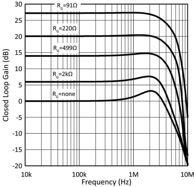
**Figure 10: Small Signal Closed Loop Phase (Gain)**
